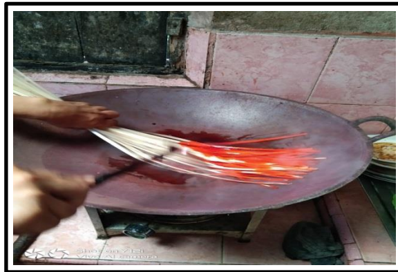
Gambar 4.4 Proses pewarnaan bambu
